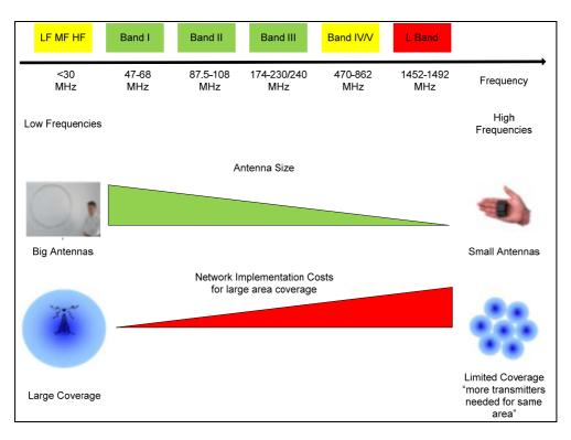
Figure 1: Characteristics of frequency for radio broadcasting antenna size and network costs
